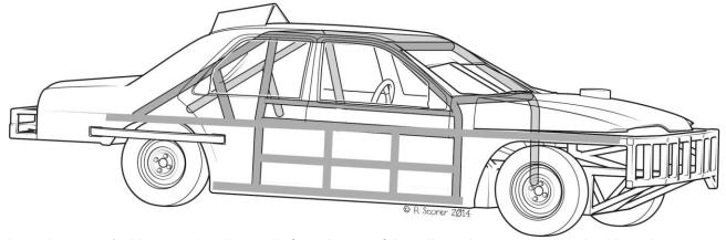
in a criss-cross fashion, running diagonally from the top of the rollcage hoop at the driver's side to the chassis on the passenger side and vice-versa.
